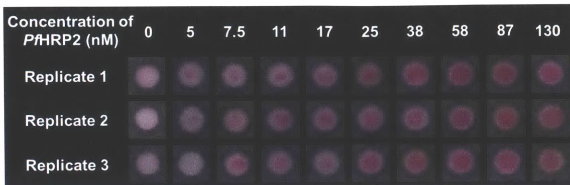
Figure 8-4 Colorimetric readout of the PfHRP2 protein in plasma after plasma separation in the microfluidic device, in undiluted blood.
