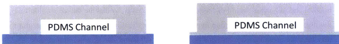
Figure 3-1 A cross-sectional view of a PDMS-defined channel bonded to a microscope glass on the left. On the right, is the final approach used for this system, where a PDMS-layer is spin-coated onto the glass and then a PDMS piece defining the channel is bonded. This improvement minimized corner bubble entrapment.
