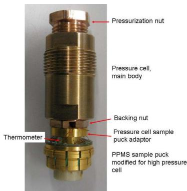
Figure 2.8: Setup of hydrostatic pressure cell. Adapted from [52].
