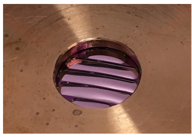
Figure 35. Top: transmission of silicon nitride windows in comparison to mylar. The expected axion spectrum is also shown. Bottom: a 300 nm silicon nitride window under 1500 mbar pressure.
