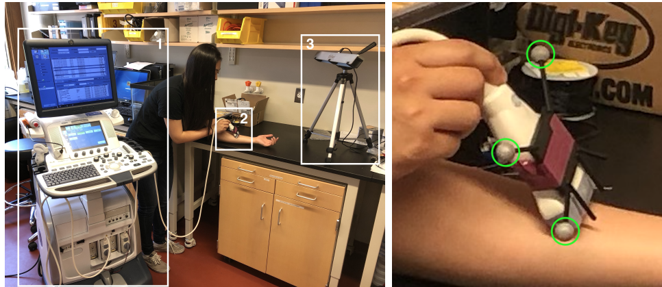
Figure 2-2: (Left) Data collection setup. (1) GE LOGIQ 9 ultrasound machine, (2) Ultrasound probe with Optitrack sensors attached, (3) Optitrack camera. (Right) Close-up image of the ultrasound probe. The Optitrack sensors are circled in green.
