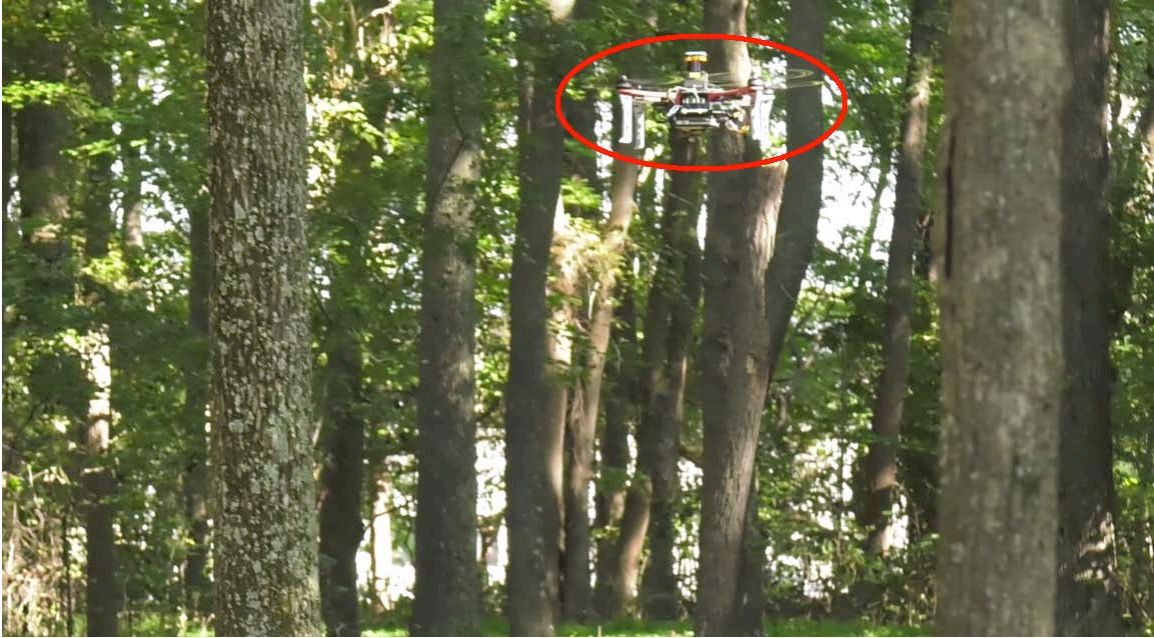
Figure 5-16. Single UAV autonomous exploration at NASA LaRC. The vehicle (highlighted in red) performs landmark-based SLAM based on detected trees in order to estimate its position within the forest.
