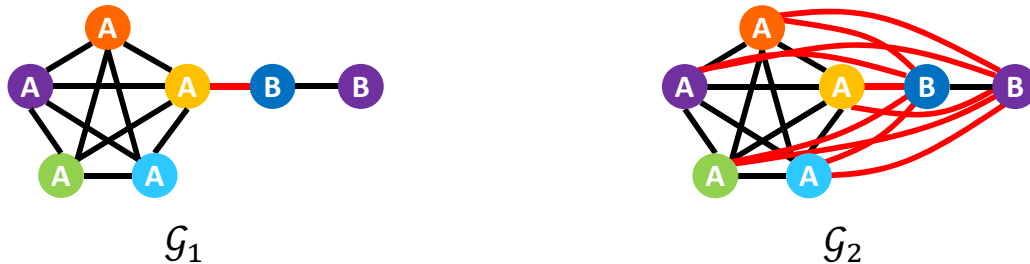
Figure 5-7. Evaluating the performance of cycle-inconsistent solutions (e.g., \mathcal{G}_1 ) for clique-centric applications must be done after completing the connected components of the association graphs (i.e., for the transitive closure \mathcal{G}_2 ). Even a single incorrect edge (drawn in red) may have catastrophic consequences in clique-centric applications.
