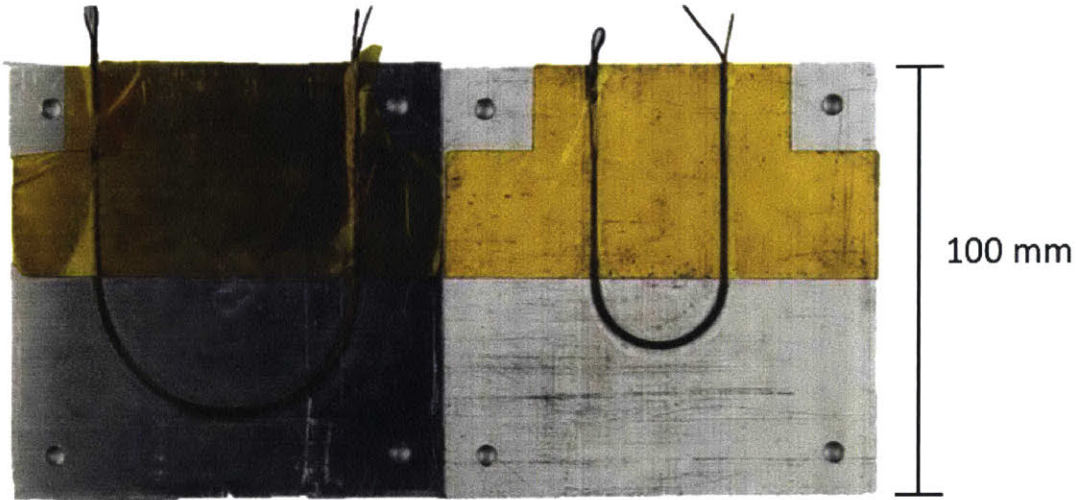
Figure 3-11: Fixtures used to thermally bond the polyethylene sheets. Two polyethylene sheets were clamped against the fixture and current was run through the nichrome wires briefly.
