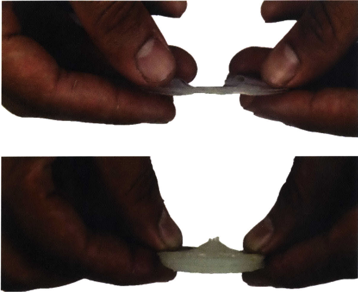
Figure 3-10: Thickness of molded (bottom) and bonded-sheet bellows. Molded bellows had a minimum thickness of 5 mm, while the bonded-sheet bellows had a sub-millimeter thickness
