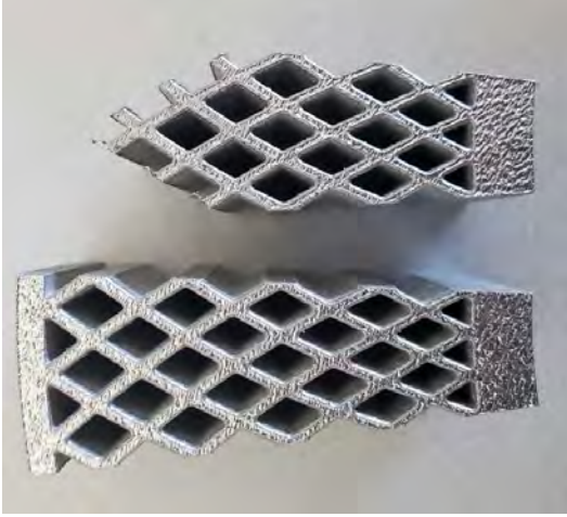
Fig. 11 Heat exchanger sample sections for surface metrology assessment
