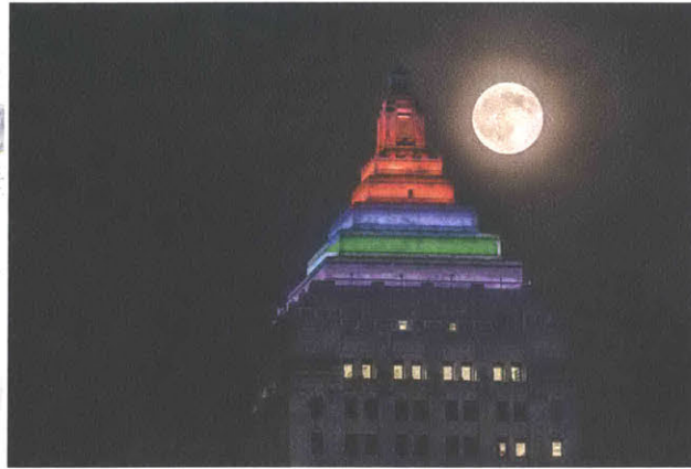
The KDKA-TV Weather Beacon. The Gulf Tower, Pittsburgh, PA. Weather information with floor by floor breakdown. 39th floor: wind speed; 40th floor: humidity; 41st floor: precipitation; 42nd - 44th floor: temperature. (DiCello, 2016)
