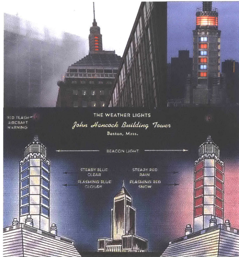
The Weather Lights. Messages conveyed by the column of lights atop the Berkeley Building (The old John Hancock Tower), Boston, MA. Steady blue means clear view, flashing blue means cloudy, steady red means rain, and flashing red means snow. When the Red Sox broke The Curse and won the 2004 World Series, the light flashed red and blue for the first and only time in its 60-year history (Grant, 1973)
