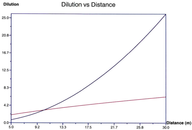
Figure 7.11: Dilution ratio \frac{C_0}{C_m} if the bypass flow were infinite (red) and if there were no core flow (blue) (drawn for 100% Power)
