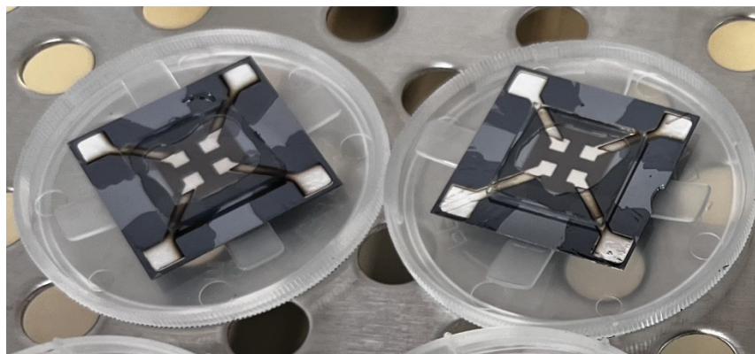
Figure 6-3. Optical image showing the top surface of the silicon-tetracene heterojunction solar cells.
