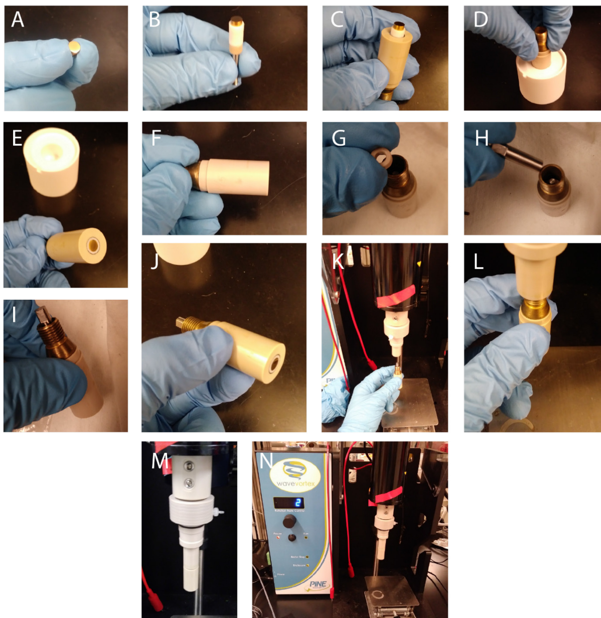
Figure A-B3. Insertion of prepared disk into RDE assembly. A) Polished Au disk. B) Disk in PTFE casing at the rotator shaft tip. C) Assembly in (B) inserted into the outer PEEK shroud. D) Pushing down the assembly in (C) to properly seat the Au disk into the PEEK shroud. E) Image of the result of proper seating. F) Side-profile image of the same. G) Dropping a plastic spacer into the back of the assembly. H) Screwing in the disk contact stud to enable electrical connection to the working electrode. I) The electrode tip assembly, ready to insert onto the rotator shaft. J) The electrode tip assembly from a different angle. K) Preparing to insert the electrode tip into the rotator shaft. L) Seating the electrode assembly into the rotator & screwing in. M) Final assembly, including gas-purged bearing attached to rotator shaft. N) Wider view of final assembly, now ready to use.
