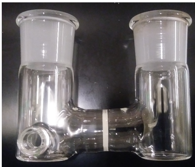
Figure A-B1. Photo of H-cell used in electrochemical experiments. Custom cell by JamesGlass.
