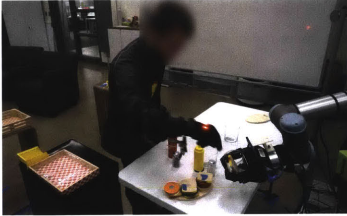
Figure 5-3: The robot delivering the required ingredient to its human teammate.
