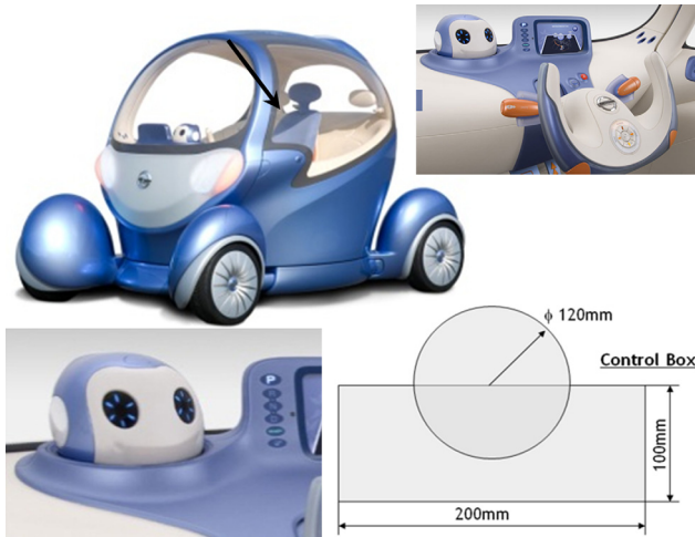
Fig. 1 Nissan PIVO, detail of RA prototype on dashboard [1] and maximum admissible dimensions specified by Nissan
