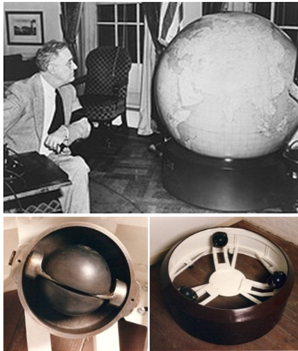
Fig. 3 Top: “President Roosevelt and his globe,” 1942, photo courtesy of FDR Library; bottom: support base and mechanism detail showing ball rotating in swiveling cup, photos courtesy of Sylvia Sumira
