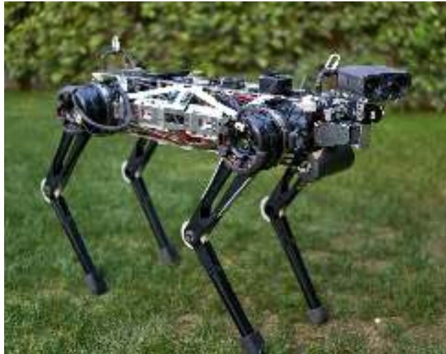
Fig. 1: MIT Cheetah 3. The MIT Cheetah 3 quadruped robot platform is an electrically powered robust robot capable of untethered 3D locomotion in uncertain terrains.
