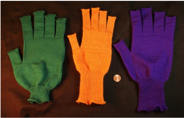
Figure 23: Three glove variants. The green one took multiple attempts because of the complicated tension requirements associated with continuous cross patterns.
