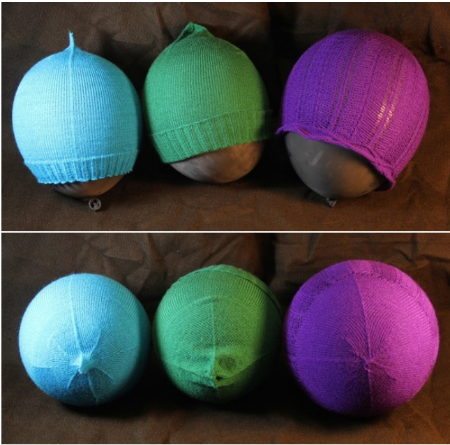
Figure 21: A reference beanie on the left and two customized beanies on its right. The rightmost one required a few passes to adjust the lace pattern and its tension.
