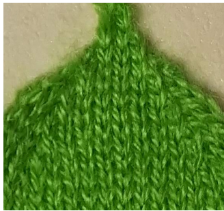
Figure 24: Standard shaper programs: (left) uniform distributes the increases and decreases uniformly, (right) center accumulates them in the center of the course. Notice the visible seam in the center. At the top are program illustrations for M = 10, N = 14 (these numbers are here for illustration, they vary for every row in a real knitting structure). At the bottom are the bed layouts and the knitted results for a flat triangular sheet.
