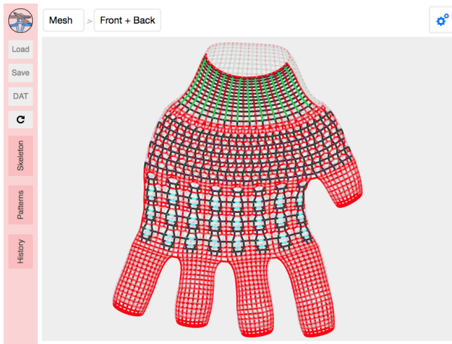
Figure 7: Force-layout simulation to preview the impact of the yarn stress forces on the final shape.
