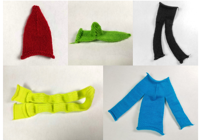
Figure 17: The individual garment pieces from Figure 1. The scarf uses a single-sided part that would curl on itself by default. Thus we used simple 2 by 2 ribs to keep it flat.
