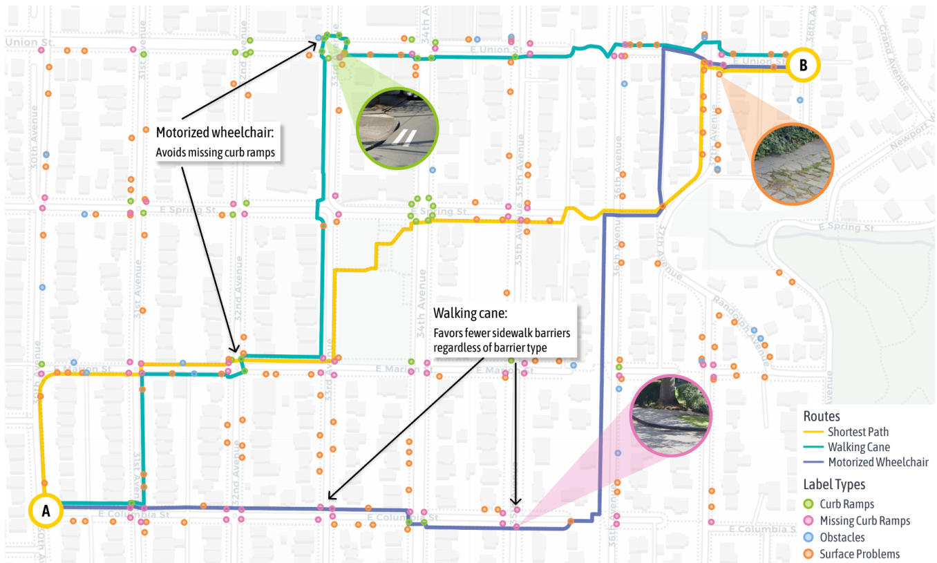
Figure 14: Routing application using OSMnx to generate routes between A & B based on our survey data. Yellow route shows the absolute shortest path; teal shows the route for walking cane, this route favours fewer sidewalk barriers regardless of category; purple shows the route for motorized wheelchair, this route avoids missing curb ramps at all costs. When hovering over the labels, users can see what the sidewalk issues look like in streetview.
