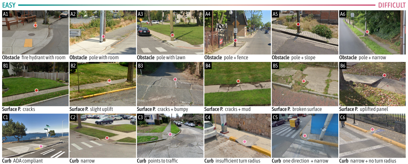
Figure 10: Image comparison result for subcategories of “fire hydrant and poles” (images A1-A6), “cracks and height difference” (images B1-B6), and “curb ramps” (images C1-C6). The images are ordered from left to right based on their Q score. For “fire hydrant and poles”, all mobility groups ranked in the order of A1 to A6 expect cane user group reversed the order of A5 and A6. For cracks and height difference”, different groups varied slightly on their rankings for B2/B3 and B5/B6. For “curb ramps”, different groups varied slightly on their choices for C3/C4 and C5/C6. See the full Q score rankings for each group in the Appendix (Figure 10).
