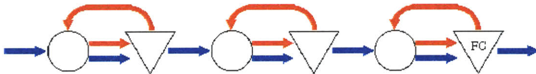
Figure 7: - Kanban control. Movement of parts shown in blue, circulation of kanbans in red. Machines are shown as circles and buffers as triangles. The last buffer is the finished goods (FG) inventory. 28
