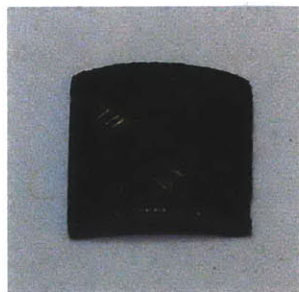
(a) Triplex thermal diffusivity square. Concavity facing down.
