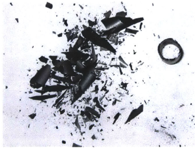
(b) Monolith only sample T-2 after hoop test. Catastrophic brittle failure.
