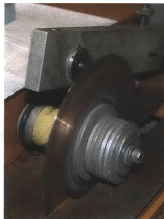
(b) Diamond-coated blade and clamp mounting arm.
