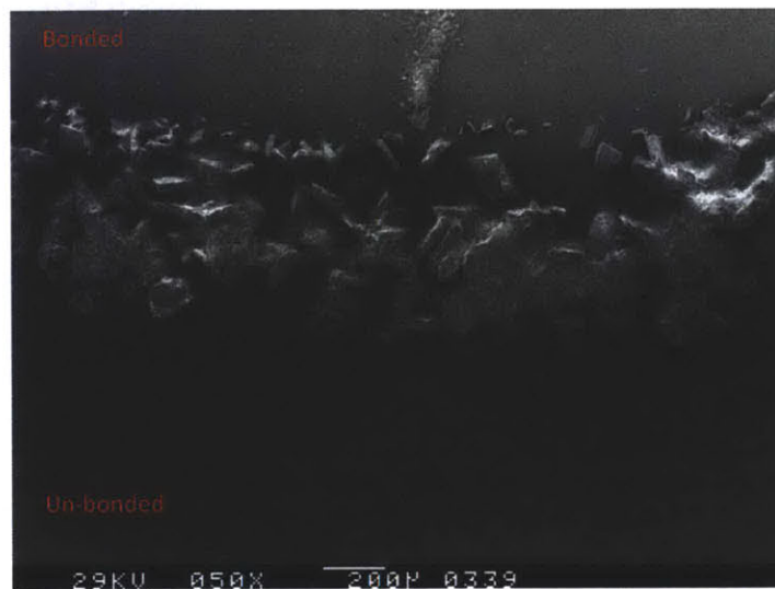
Figure 4.10: Rhombohedral calcium aluminate crystals on the bondline between the bonded and un-bonded regions of sample 5A.
