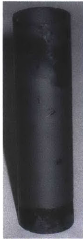
(a) 25-2 before hoop testing. The weave pattern is not visible through the thicker EBC.
