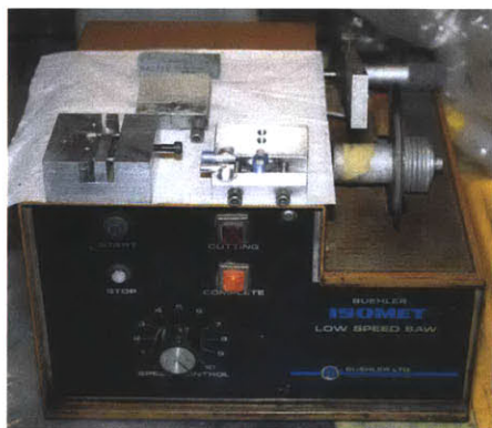
(a) Buehler Isomet saw with three sample clamps.
