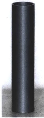
(a) Monolith only sample T-2 before hoop test.
