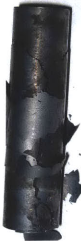
(c) 25-2 after failure displaying "v"-shaped cracks at both ends and an axial crack connecting the two ends.
