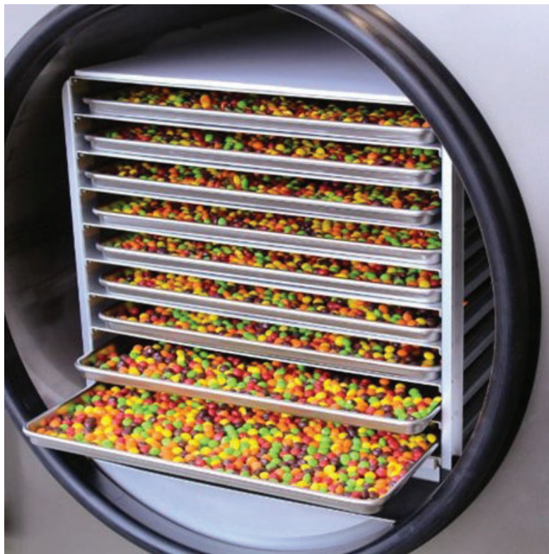
Figure 1.9: Bulk lyophilization machines like the one shown here are often used in food freeze drying, where specific mass requirements are not as strict as they can be in pharmaceuticals. Image from [21].
