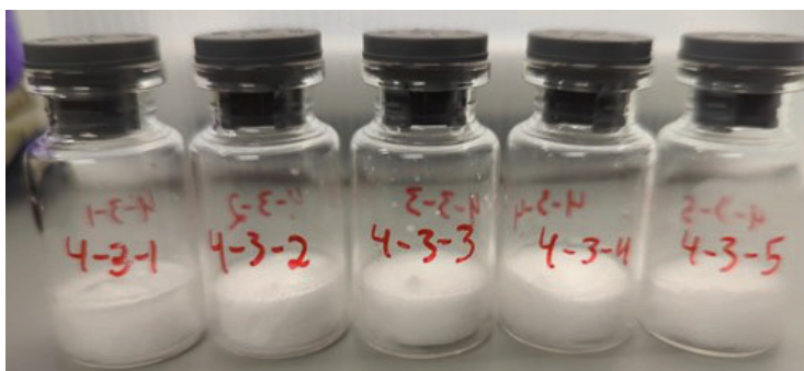
Figure 5.1: Once a solution has gone through the drying process of lyophilization, the liquid is removed from the product to leave behind a solid crystalline cake.
