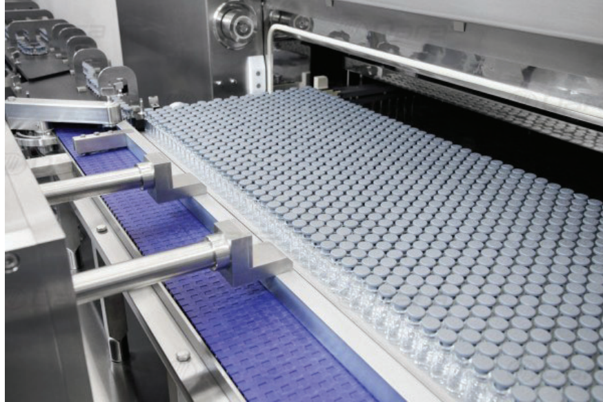
Figure 1.8: A commercial freeze dryer loading one shelf in a freeze drying batch run. These commercial systems include thousands of vials per batch. Image from [20].
