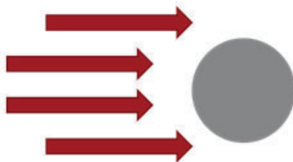
Figure 3.3: The vials in the forced gas convection chamber can be modeled as cylinders in crossflow.
