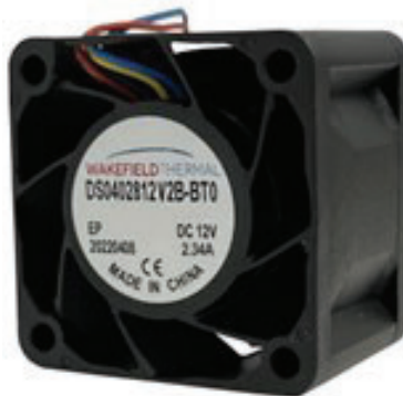
Figure 3.6: The muffin fans used to generate the gas flow in the cooling chamber are 40mm x 40mm x 28mm muffin fans. These fans generate gas flow locally at the cooling chamber inlet, localizing the flow generation to each individual module.
