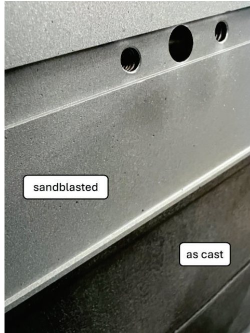
Figure 6.6: The stator pocket in the machine chamber and the Planar Motors stator are sandblasted in preparation for vacuum sealing. This sandblasting increases the adhesion between the injected vacuum sealant and the two components, improving the vacuum seal fidelity.
