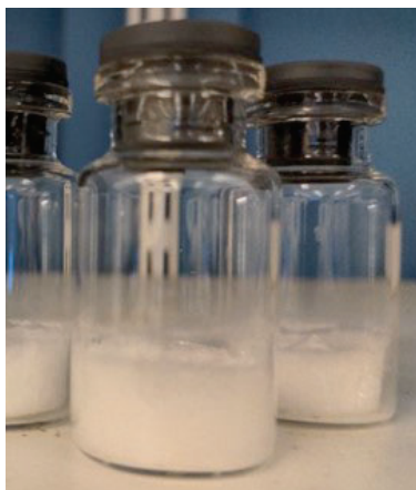
Figure 1.5: The representative lyophilized cakes shown are examples of what the product looks like after undergoing the lyophilization process.
