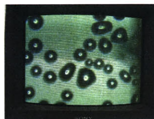
(b) Microbubbles observed in microscope upon injection of ethanol in fluid cell
