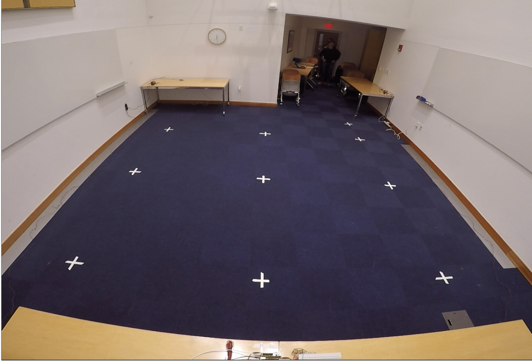
Figure 6-2: Our developed system was deployed in an indoor localization environment at MIT. The white crosses on the floor are used to recreate each target’s ground truth tracks.
