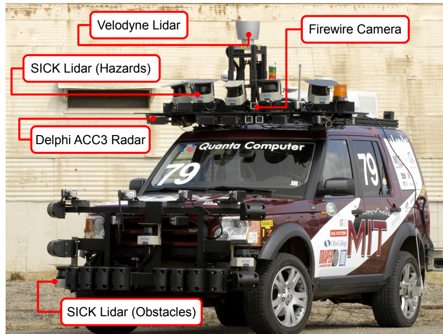
Figure 9: MIT's 'Talos', a Land Rover LR3 featuring five Point Grey FireFly cameras, 15 Delphi ACC3 radars, 12 Sick LMS-291 lidars and a Velodyne HDL-64 lidar.
