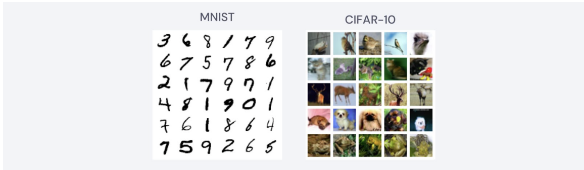
Figure 5-1: Benchmark datasets used in image classification. MNIST contains 60,000 black-and-white handwritten digits. CIFAR-10 is a collection of 60,000 images spanning 10 categories.
