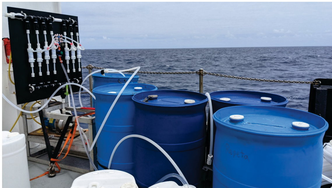
Figure 5.1: Custom large volume POM concentrator used on PARAGON I to collect SPM samples. The seven hollow fiber filters (white) retain particles larger than 0.1 \mu\text{m} .
