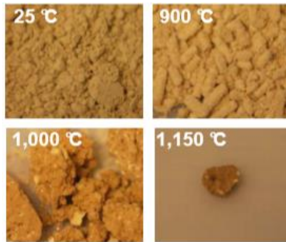
Figure 2-15: The morphology of ash samples shown at various ambient temperatures, from 25 to 1,150 Celsius. It is plainly evident that ash sinters and shrinks into high-density agglomerates as temperature rises [23].
