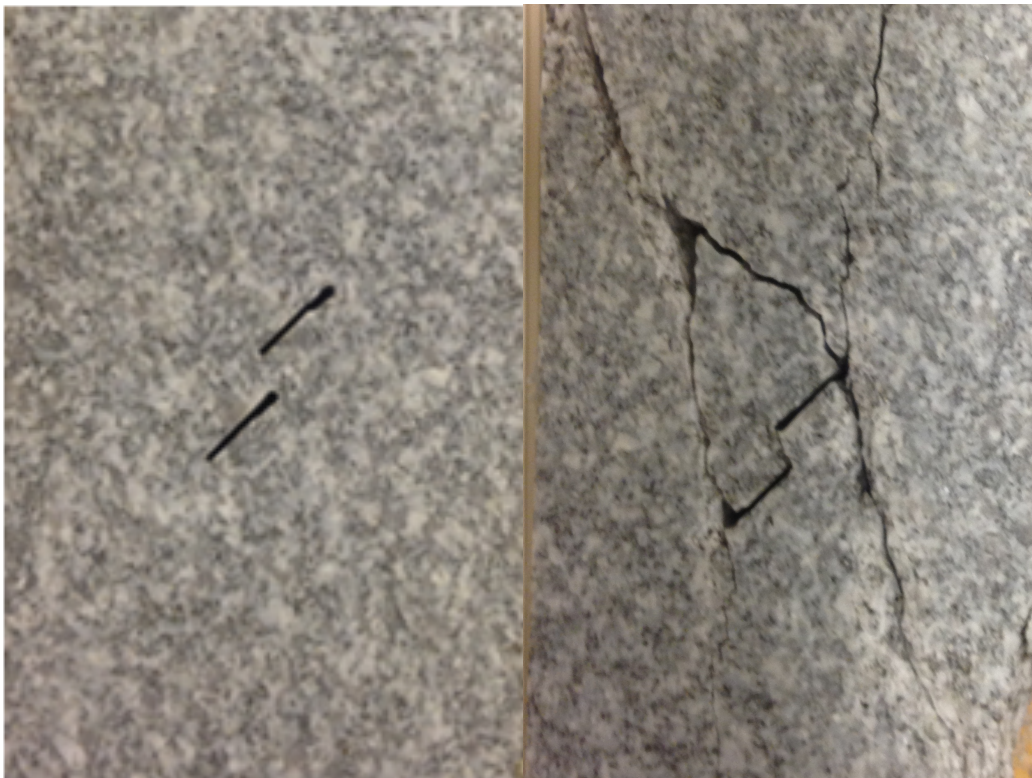
Figure 14: Photo of the AE-GR-a-45-60 specimen before and after the test
