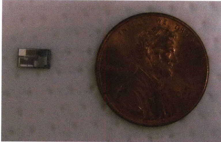
Figure 6.6 Small size Si ROIC chip (3 mm \times 5 mm) for monolithic integration.
