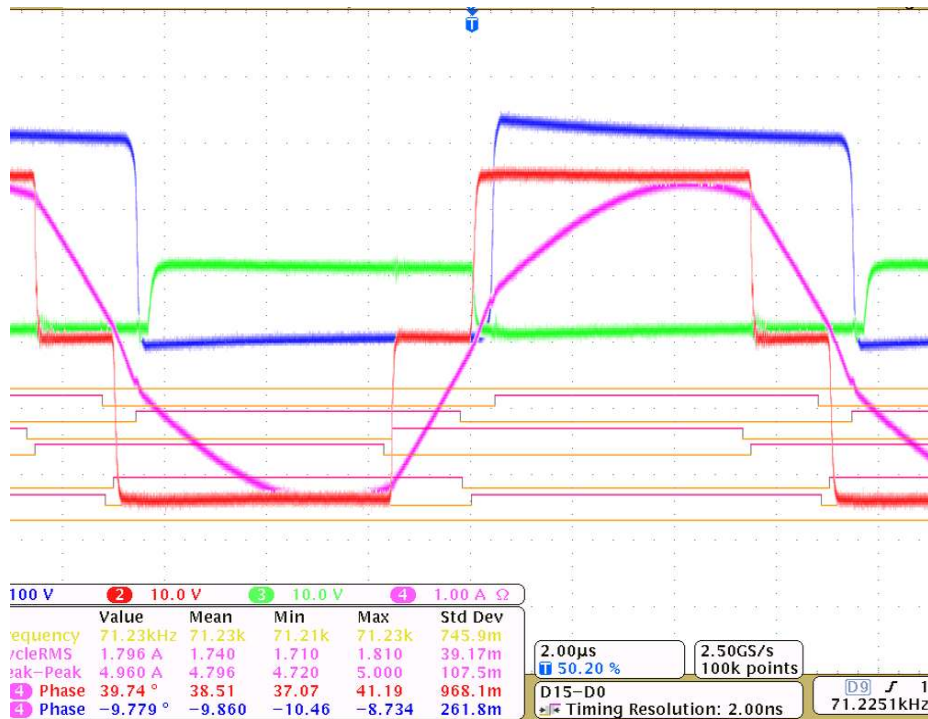
Figure 5.11: Typical inverter waveforms. 250W is outputted from 25V in to 305V. -v_{CC} is in blue, i_x is in purple, v_{FB} is in red, v_{gs, FH} is in green, The non flat top of blue is an artifact of the differential probe used to take the measurement.
