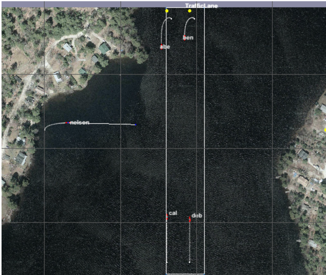
Figure 3-10: Snapshot of vehicles and environment rendered by pMarineViewer. Nelson is ownship traveling west to east through a traffic lane. Nelson’s goal point is a yellow point on the middle right side of this picture. The boundary of the traffic lane and the vector that points from Nelson to the transition are both produced by the DensityCount behavior
