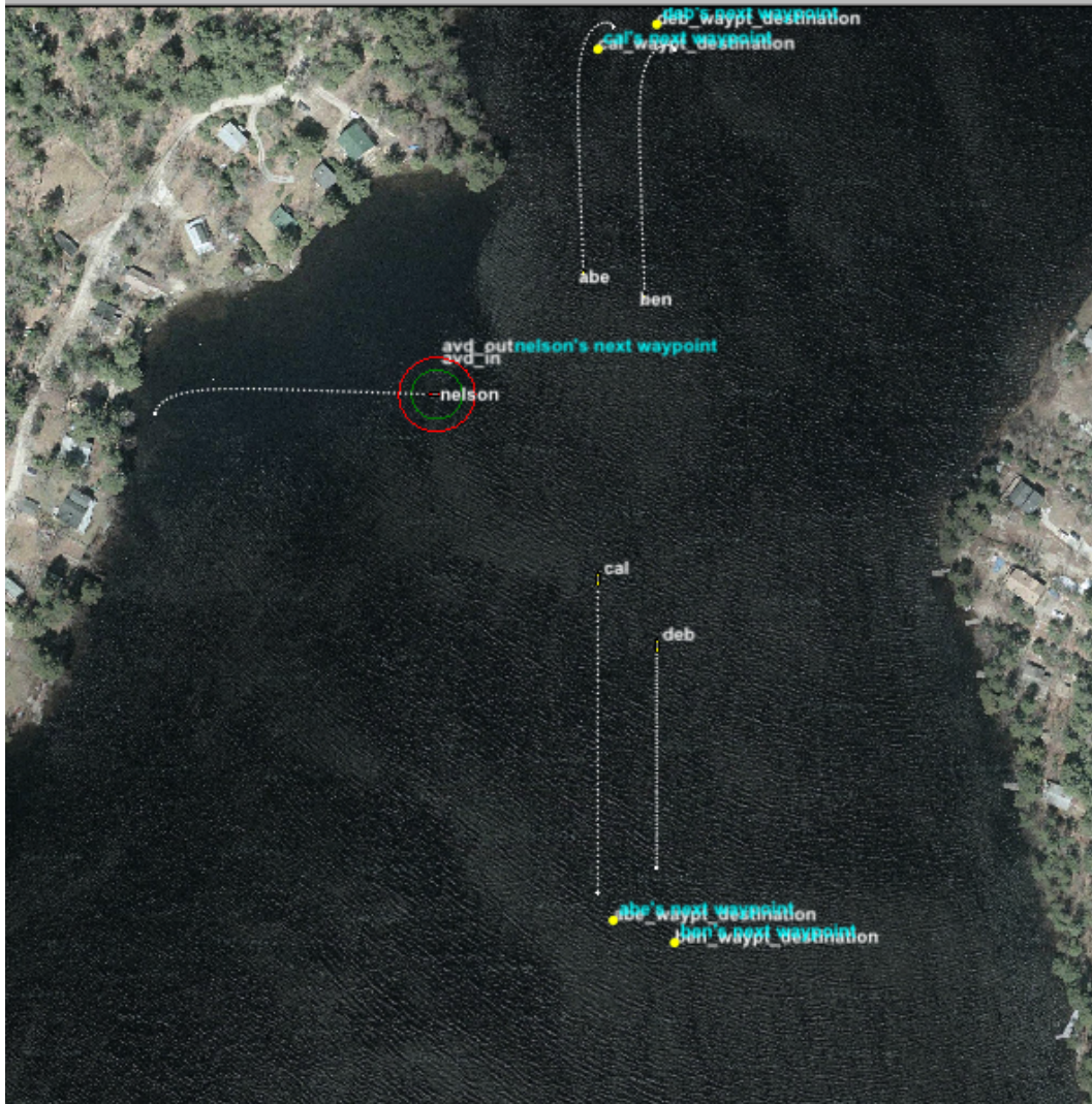
Figure 4-4: Snapshot of a control group run. All vessels follow pre-planned waypoints and speed. No collision avoidance is conducted.
