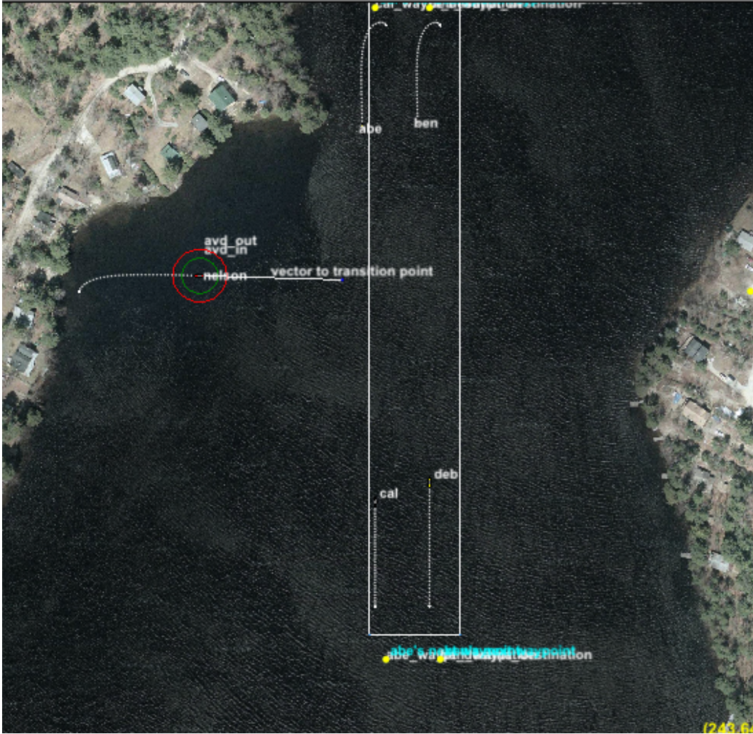
Figure 4-5: Snapshot of a experimental group run. All vehicles follow pre-planned waypoints and and speed. No collision avoidance is conducted.
