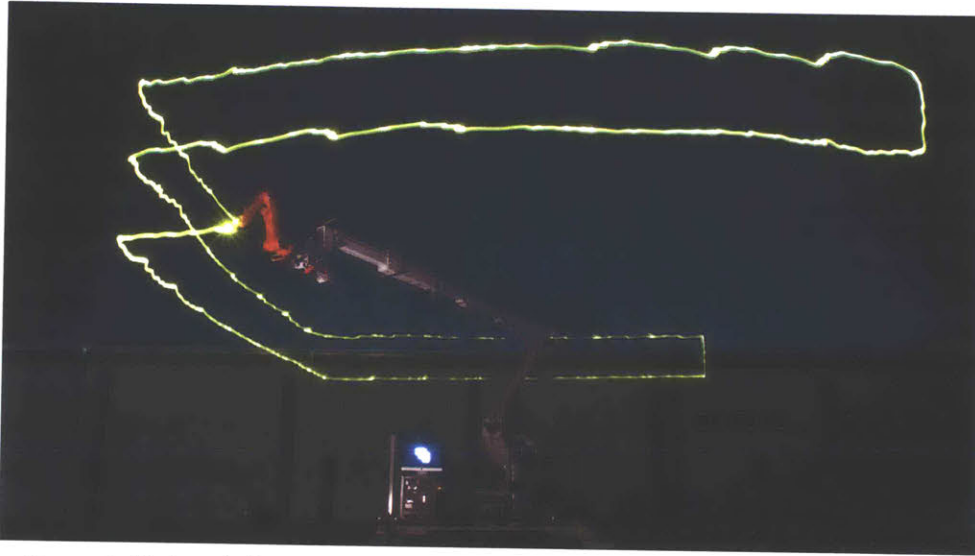
Figure 6: Light painting using control system preceding FK, IK, and trajectory generation optimizations. Points were specified roughly 1 m apart and controlled in joint space, which results in the “waves” between points.
