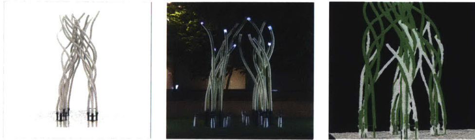
Figure 41: The pre-designed structure is shown on the left (designed up to 10 m tall), and the final structure in the middle (roughly 4.5 m), and photogrammetry of the actual structure overlaid on the designed structure on the right, it is clear that drift occurred, estimated at about 0.5-1 m or so over the entire length. Photogrammetry credit to Silas Hughes.
