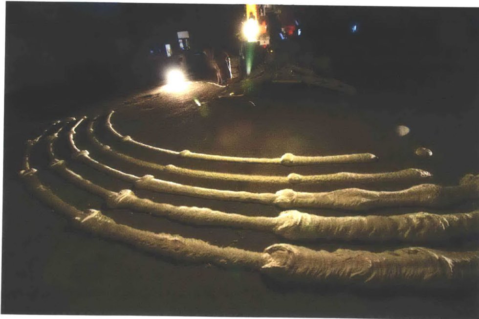
Figure 13: Many empirical tests were performed to find mappings between Cartesian speed of the end-effector, the distance of the nozzle from the print height, and the spray nozzle settings, and their effects on bead size and overall material deposition rate.
