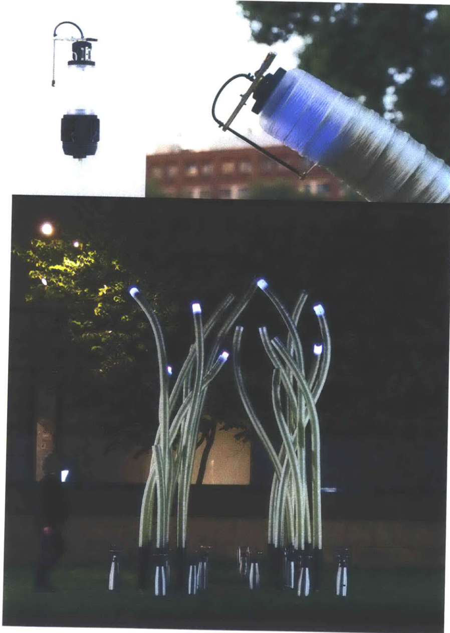
Figure 22: (Top-left) shows a single Fiberbot, (top-right) shows a single Fiberbot as it is winding a fiberglass tube, and (bottom) the entire Fiberbot system, using 16 robots, as it creates a large, "woven" architecture in parallel.
