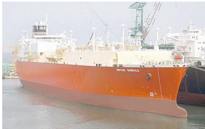
Figure 5-7: LNG-fueled LNGC dual fuel diesel electric vessel (BP Shipping). From the “Gem” series of BP Shipping’s LNGCs, the British Emerald is a dual fuel diesel electric vessel selected for its relative clean environmental performance to diesel LNGCs (Society of Petroleum Engineers).
