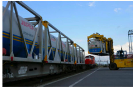
Figure 5-11: LNG mobile storage containers for intermodal transport of the fuel. LNG mobile storage containers of standard ISO size. The picture on the left is transportation of the filled container via truck, the picture on the right is the same ISO container being loaded onto a rail car (Rostock, 67). The picture below is an extension to the possibility of these same intermodal containers loaded onto a small container vessel to transport port-to-port (SGL1, 5).
