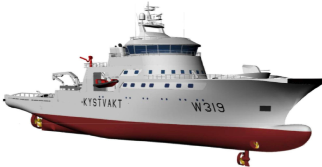
Figure 5-12: LNG-fueled coast guard vessel (Norway). LNG-fueled design of Norwegian Coast Guard vessel. The vessels will be supplied gas from Barents NaturGass AS (Skjervheim, 21). The vessels are powered by Rolls-Royce Bergen K gas engines and capable of 40 knots (Ingjerd).
