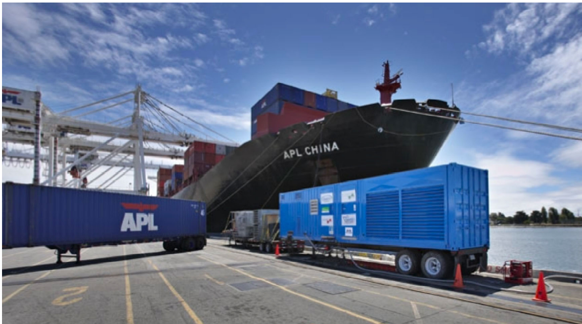
Figure 6-1: LNG cold-ironing in the United States (Port of Oakland). LNG exists at ports in the United States that do not have an LNG receiving terminal. This picture shows shore-side clean power being provided to the APL China via LNG cold-ironing from a mobile containment unit at the Port of Oakland in the summer of 2007.
