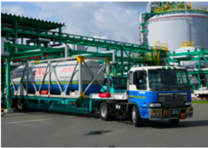
Figure 5-11: LNG mobile storage containers for intermodal transport of the fuel. LNG mobile storage containers of standard ISO size. The picture on the left is transportation of the filled container via truck, the picture on the right is the same ISO container being loaded onto a rail car (Rostock, 67). The picture below is an extension to the possibility of these same intermodal containers loaded onto a small container vessel to transport port-to-port (SGL1, 5).
