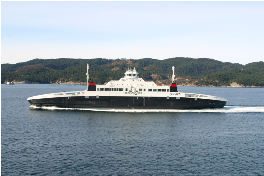
Figure 5-5: LNG-fueled ferry vessel (Norway). A Fjord1 LNG-fueled ferry with a symmetrical design for ease of loading and unloading of passengers along its Norway routes (Fjord1).
