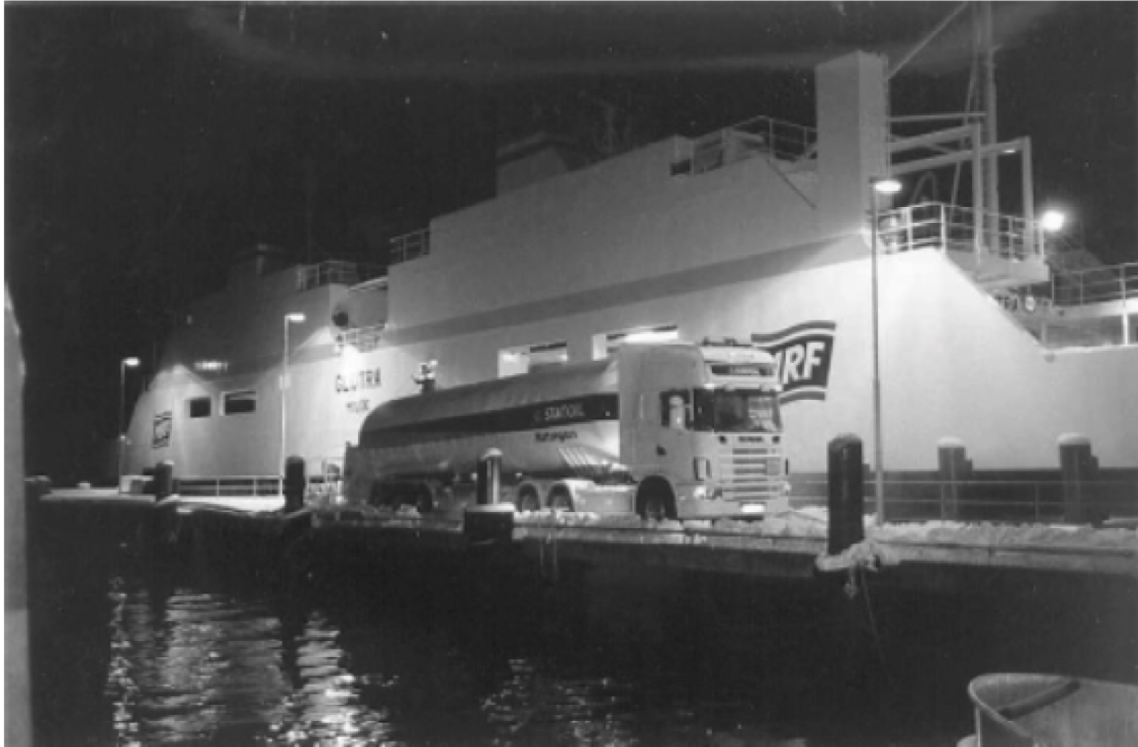
Figure 5-10: LNG-fueled ferry vessel bunkering via tanker truck (Norway). The DFDE Fjord1 ferry vessel, Glutra , is bunkered by a tanker truck at berth each evening (Einang1).
