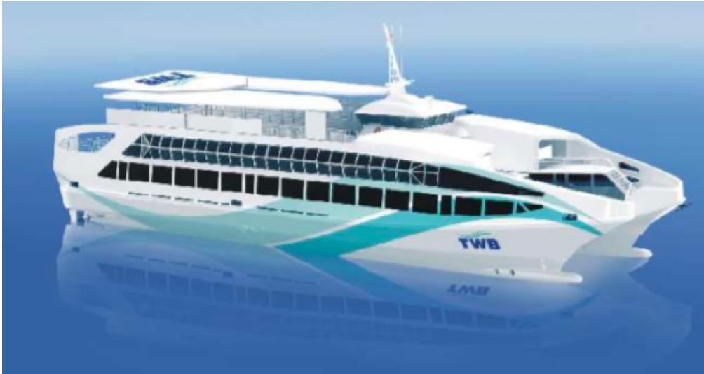
Figure 5-6: LNG-fueled RoPax vessel (Brazil). The design concept for the new dual fuel diesel electric (DFDE) catamaran RoPax vessel for TWB Group in Brazil. The vessel was launched in March 2008 (TWB).
