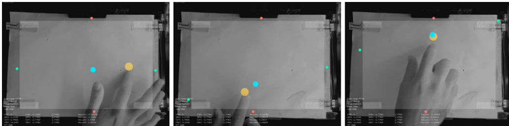
Figure 5.16: Screen capture from interface touch location in three distinct positions. Red circles refer to x_{top} , x_{bottom} positions. Green circles refer to y_{left} and y_{right} positions. Cyan circle refers to the intersection between x and y axis. Yellow circle refers to position where touch was detected.
