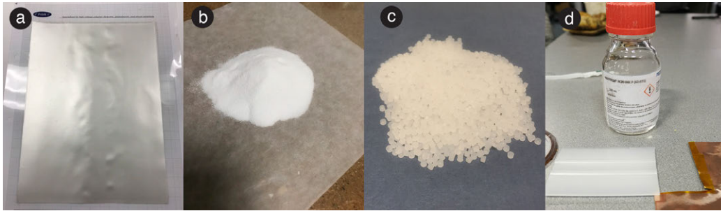
Figure 4.17: Image with types of piezoelectric materials a. PVDF poled piezoelectric film with silver ink electrodes b. P(VDF-TrFE-CFE) Terpolymer c. PVDF Homopolymer Pellets d. P(VDF-TrFE) Copolymer Resin Source: (PolyKTechnologies, n.d.)
