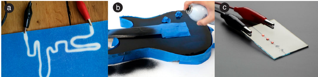
Figure 2.13: Examples of interactive inks and pigments. a. Interactive drawing with thermochromic ink (Hutton, n.d.). b. Conductive coating used for touch sensing on everyday objects (Zhang et al., 2017) c. Visual LED display applied on Indium Tin Oxide (ITO) coated on glass. (Adafruit, 2020)
