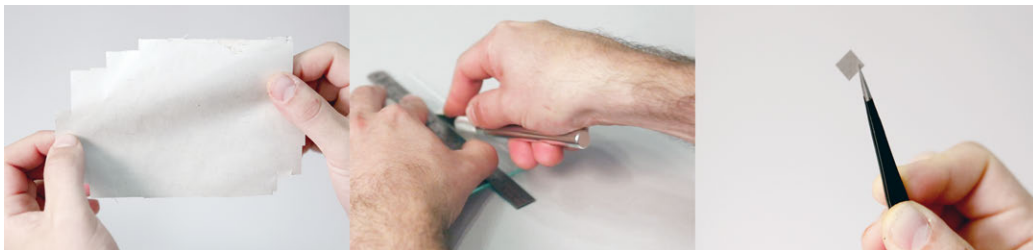
Figure 6.7: Steps for cutting the piezoelectric thin film into dices that can be laminated on paper surface.
