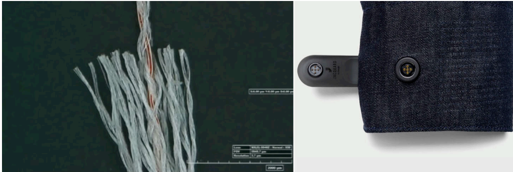
Figure 2.8: Image of Project Jacquard by Google. Left: Close-up of yarn comprised of conductive and non-conductive material. Right: Jacquard yarn woven into the cuff of Levi's jacket. Source: Poupyrev et al. (2016)
