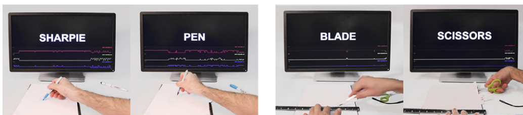
Figure 6.9: Image of laminated vibroacoustic paper demo. Left: SVM model classifies interaction between paper and writing implement. Right: SVM model classifies cutting implement.
