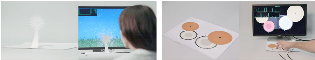
Figure 6.8: Image of laminated vibroacoustic paper demos. Left: Drumkit demo using two vibroacoustic sensors laminated on the underside of paper to detect touch interaction with printed graphics. Right: Interactive dandelion demo using wind vibration to enhance interaction with paper with graphics on screen.
