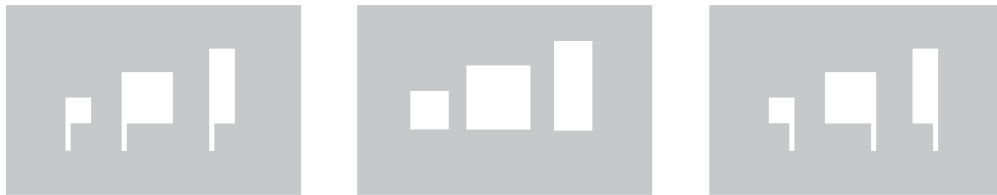
Figure 6.11: Mask designs for vibroacoustic sensor. Left: Bottom electrode. Middle: Piezoelectric layer. Right: Top electrode.
