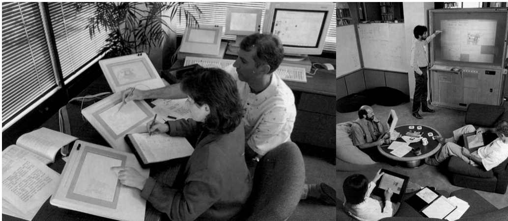
Figure 2.1: Image of Ubiquitous Computing device prototypes at XEROX Palo Alto Research. Left: Prototypes of computer scratch pads Right: Researchers at XEROX Palo Alto experimenting with prototypes of boards, pads and tabs. Source: Weiser (1991)
