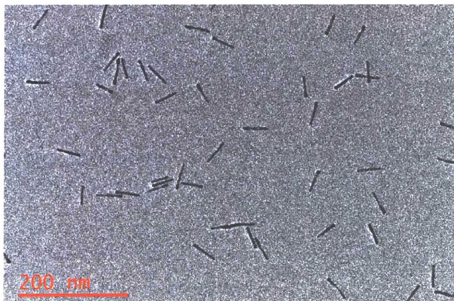
Figure S2: The TEM micrograph of the initial nanorod sample (F1)
