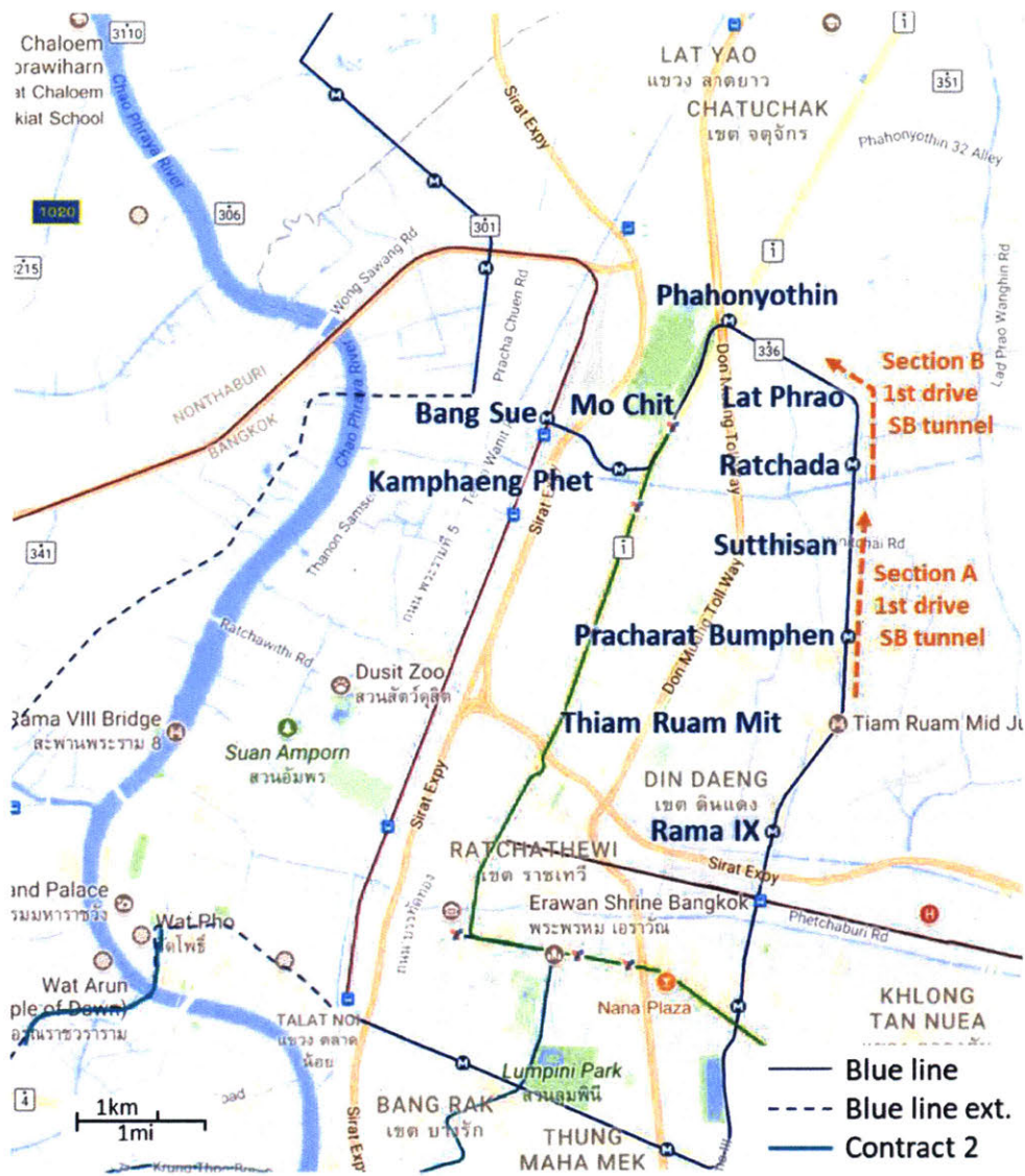
Figure 5.19 MRTA project, location of north tunnel alignment (source: Suwansawat, 2002, AECOM, 2011 and Google maps, 2017)
