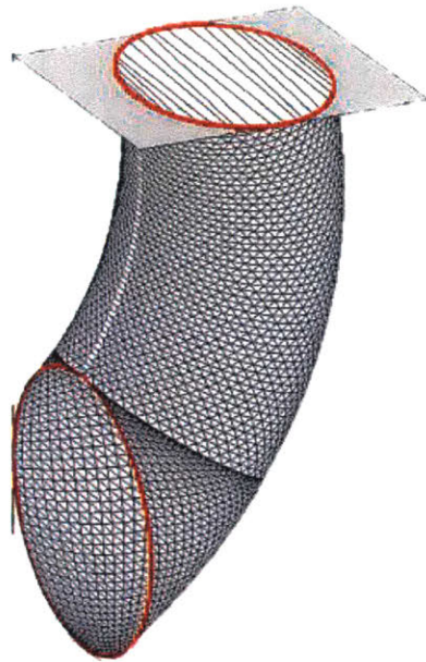
Figure 2.17 3D failure mechanisms considered for the upper bound solutions (after Mollon et al., 2011)
