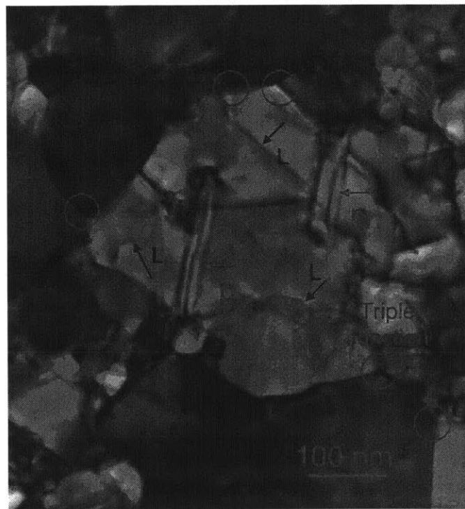
Figure A.3. Defect creation in a 45nm gold film after substantial abnormal grain growth.
