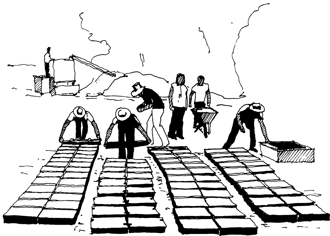
Figure 3.19 Adobe block manufacture in Peru
