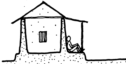
Fig. II.11. The layering technique for building earthen walls.
