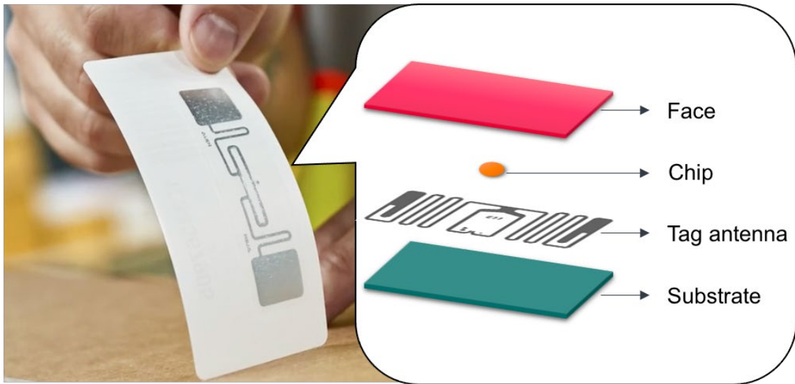
Figure 6-9: An exploded view of a typical RFID tag
