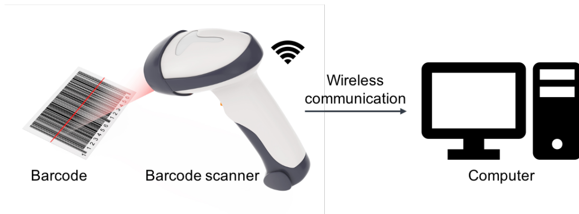
Figure 5-11: How barcode works. The scanner uses a beam of light to read the barcode comprised of parallel black lines with various widths and spaces and then send it to the computer through a wireless network.
