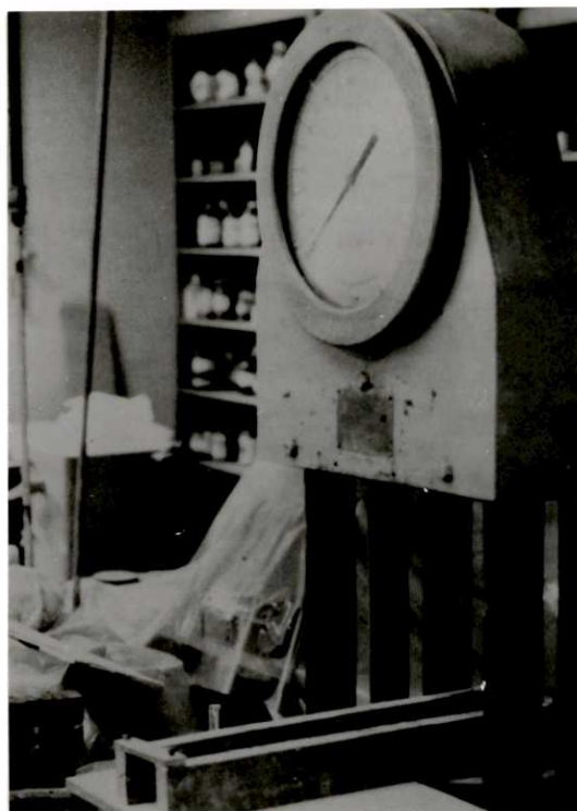
Figure 7. Photograph of hydraulic press (Watson-Stillman, 200,000 lb. maximum load) and slide track (for moving mold back and forth).
