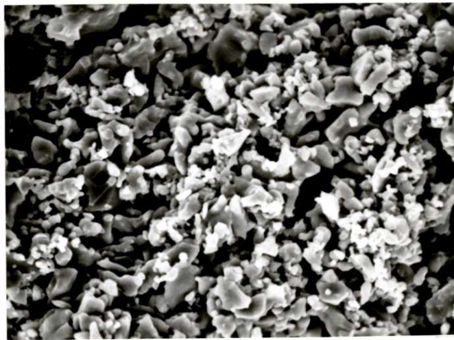
Figure 22. SEM photo of grain structure in alumina-9% magnesia, showing quite small and ragged grains and some void coalescence to cracking (Batch #12, 1175X).
