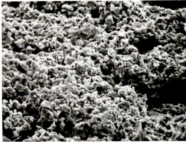
Figure 21. Evidence of void coalescence to form cracks is shown in this micrograph of alumina-9% magnesia (Batch #11, 580X), on the left and in the upper right-hand corner
