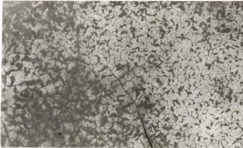
Figure 25. Photograph of surface of alumina-titania brick (Batch #24, 10 cycles, 1.7X), showing quite extensive micro-cracking.
