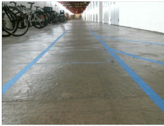
Figure 4-2: Physical setup for testing visual lane-following system. Blue lines of tape on the ground are detected by the simple visual system as lane lines.
