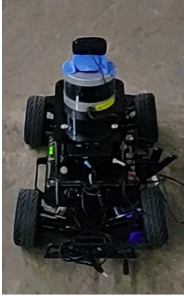
Figure 2-6: Remote-controlled robot car outfitted with LiDAR unit.
