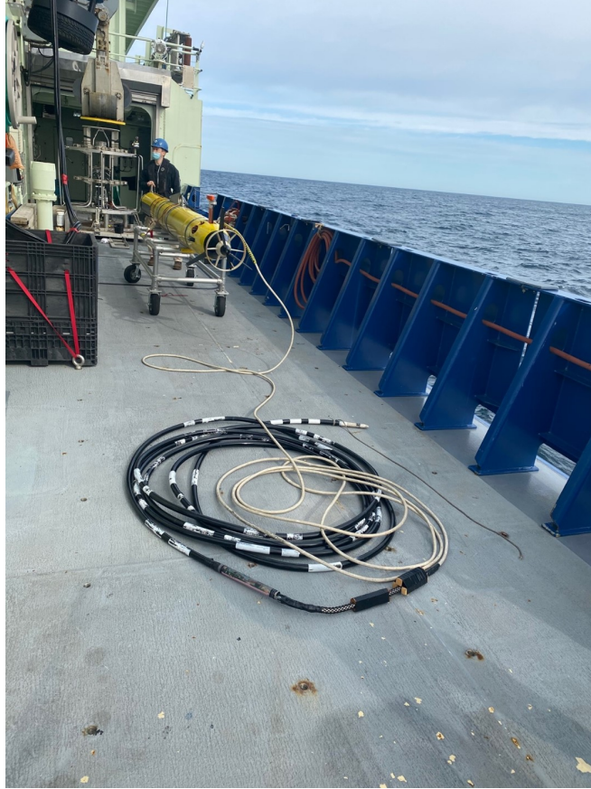
Figure 1.1: REMUS 600 and towed array used in both experiments. The towed array is 11.1 meters long and contains 16 elements.
