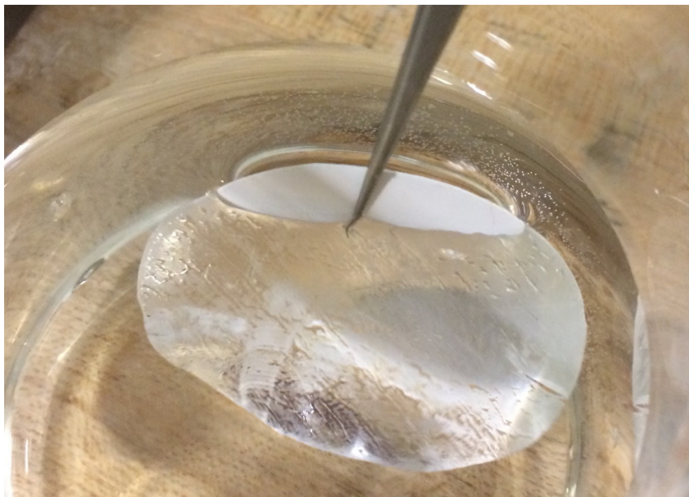
Figure 5. Photograph of submerged superhydrophobic MD membrane. The membrane appears reflective due to the air layer on the membrane surface.
